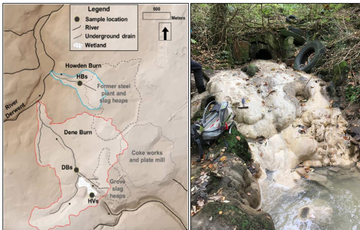
Figure 1: A map adapted from Mayes et al. (2018) showing the geography of the Consett steel works case study site (left) and a photograph showing the point of outflow of the Howden Burn from the steel works slag heaps where there is significant calcium carbonate (CaCO 3 ) precipitation.
