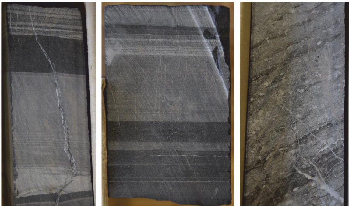
Figure 2. Core photos of lithologies from Bowland Shale Formation. Demonstrates the range of samples collected during visit the BGS core store.
