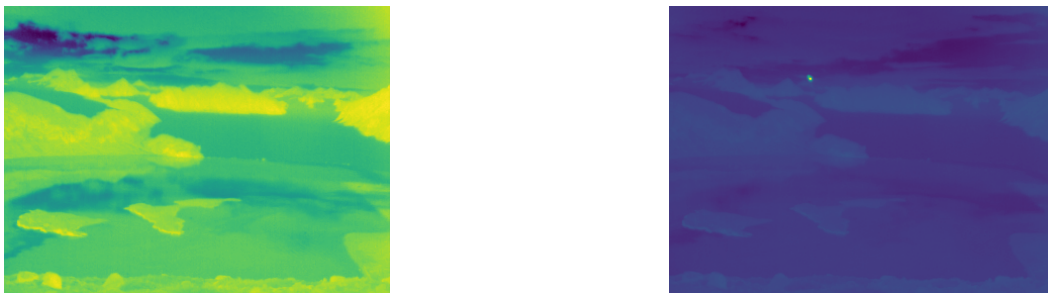
(a) If the surface of the fjord is specular, the sky is perfectly reflected at thermal wavelengths.
