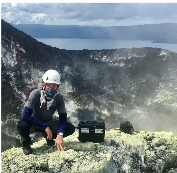
Figure 2. BTMK with MultiGAS instrument on Tavurvur's eastern crater rim. The instrument is placed directly in the gas plume and measurements are written directly to an onboard micro-SD card. Note that data could also be radioed directly to the observatory.
